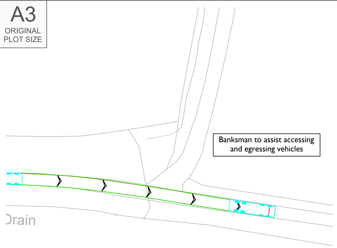
Tipper Vehicle Entering Site
